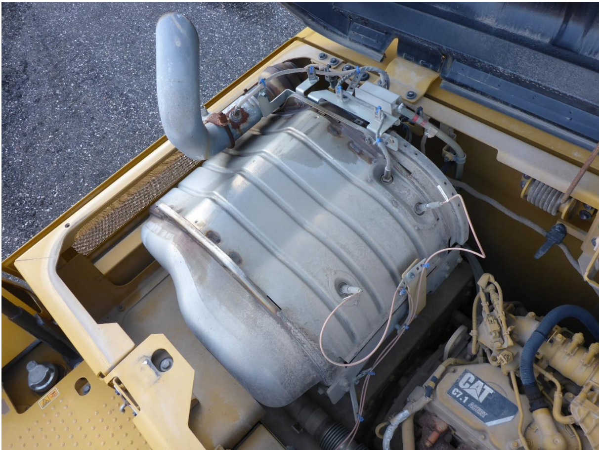
Exhaust Aftertreatment with sensors on a CAT excavator
