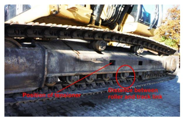
If track sag is not within the tolerance it must be adjusted. Usually the tightening works with a grease gun. If track sag is too low (chains are too tight) it needs to be adjusted as well. On most tracked excavators is a release pin mounted where grease can be left out.
